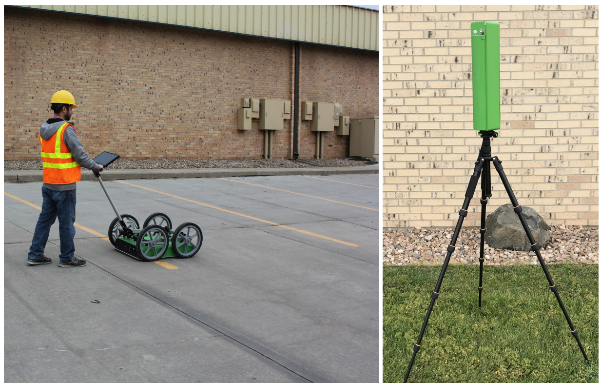
Figure 1. The Utility Scanner system with the scanner (left) and the optional GPS base station (right).
